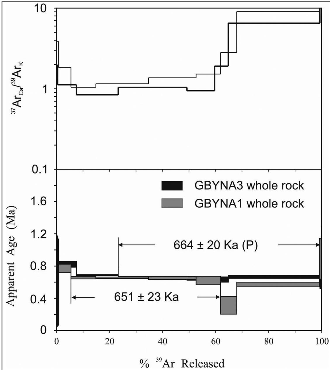
Figure 5. Ar-Ar spectra of two basalt samples.
